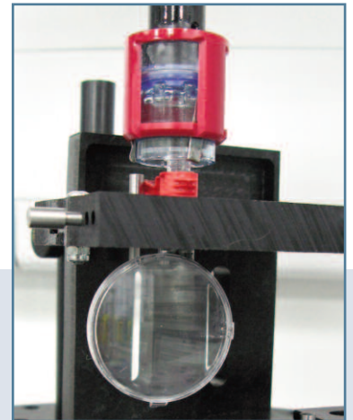
Spectacle dial presented for testing in special test fixture
