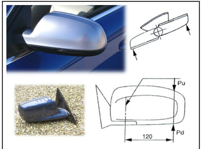
Automotive side mirror durability testing specification
