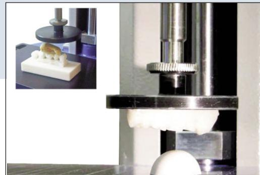
Compression and Fracture Test by Dental Model and Brittle Plaster of Paris Dome
