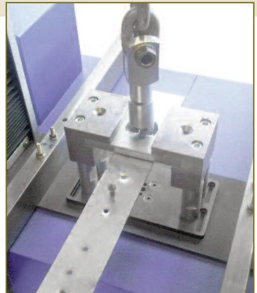
Strip fasteners under test
