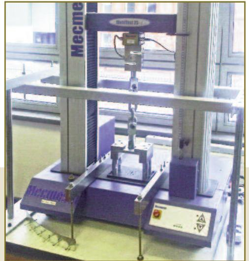
The test stand with custom-made test sample fixtures
