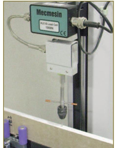
Probe shown attached to loadcell before being inserted into plasterboard sample
