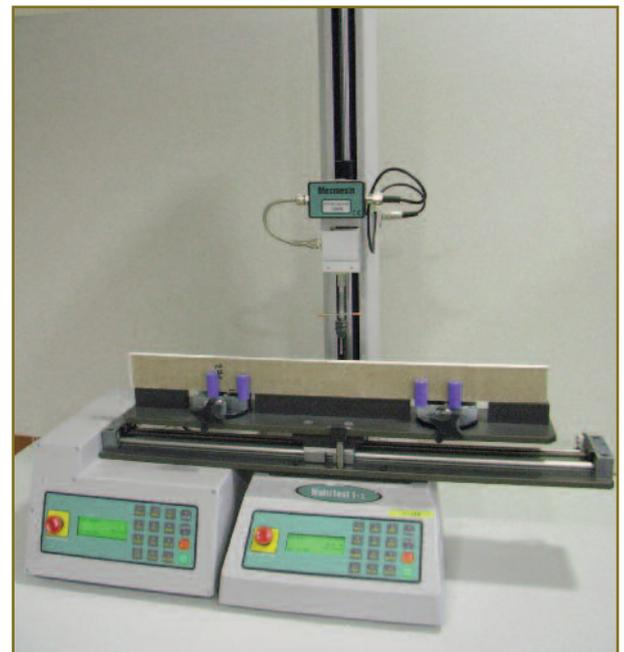
Specially constructed MultiTest-x shown with a simulated PLC indexing unit
