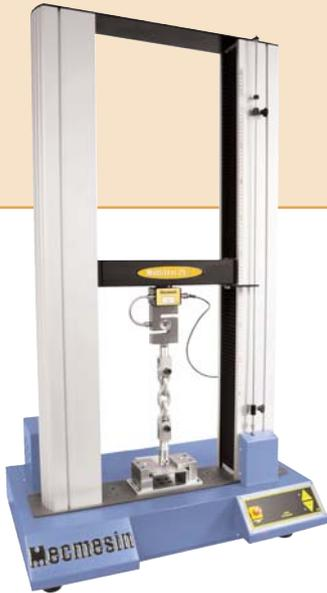
The MultiTest 25-i computer-controlled test system
